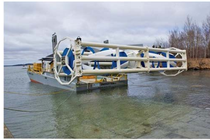
ORPC Beta Turbine Generator Unit, Eastport ME
