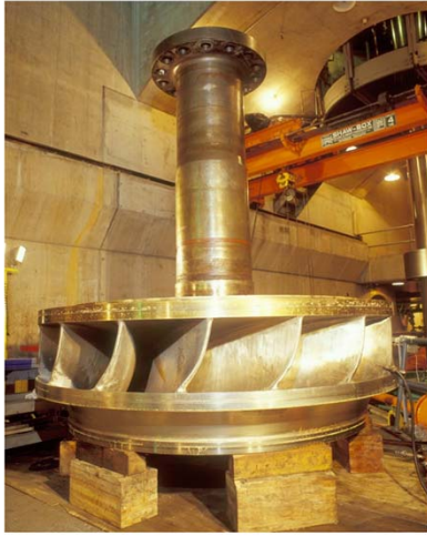
Retired turbine from Hoover Dam
