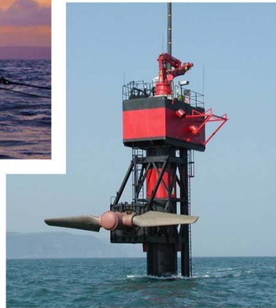
Seaflow Tidal Stream Generator
